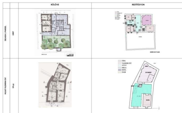
Figure 26: 581/7 and 561/12 survey and restitution projects
